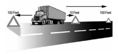
On two-lane roads carrying traffic in both directions or on an undivided highway, place warning devices within ten feet of the front or rear corners of your vehicle. Place a warning device 100 feet behind or ahead of your vehicle. Place it on the shoulder or in the lane where you stopped.
